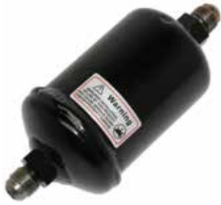
REF 143TA7600 LPG filter dia. 61,5 mm, lenght 155 mm, 3/8" SAE
