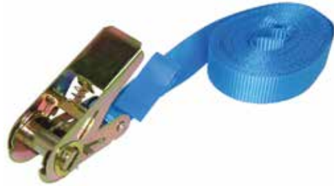
REF 105TA4855 Nylon strap fastener, for all applications length: 5 m, width: 25 mm resistance: 400 kg
