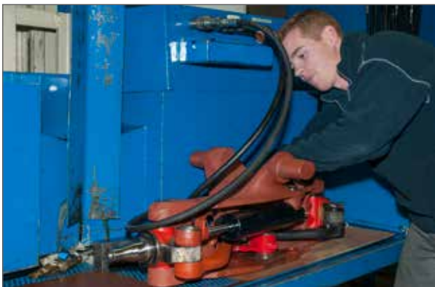
Steering cylinders tested directly on the rear axle.
